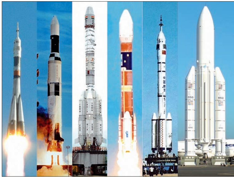
Launch vehicles around the world. From left to right, the Soyuz (RSA), the Saturn V (NASA), the GSLV (ISRO), the H2A204 (JAXA), the LM2E (CNSA), the Ariane 5 (ESA)
